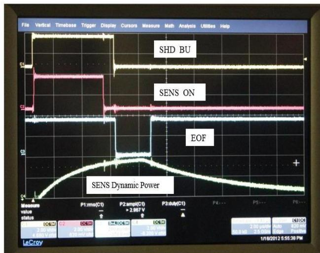
Figure 5. Dynamic power signals of DLS system-Power unit
