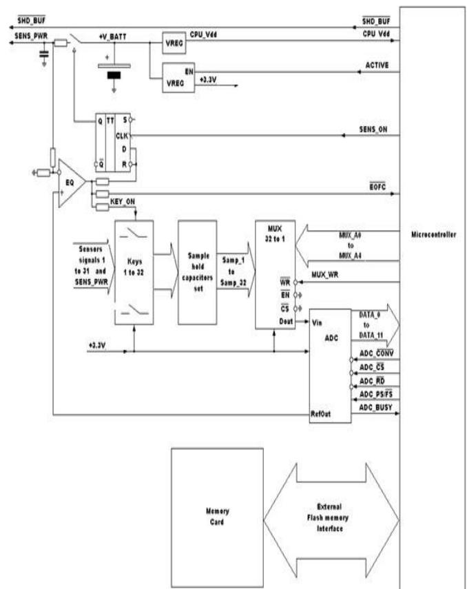
Figure. 1. Data acquisition system diagram
