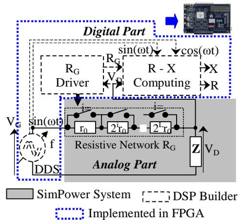
Figure 7. HIL scheme of the FVC method
