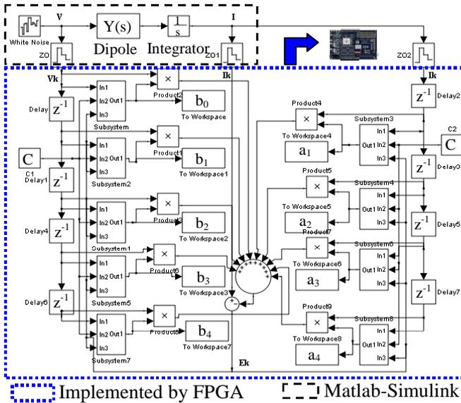
Figure 8. HIL scheme of the adaptive parametric modelisation
