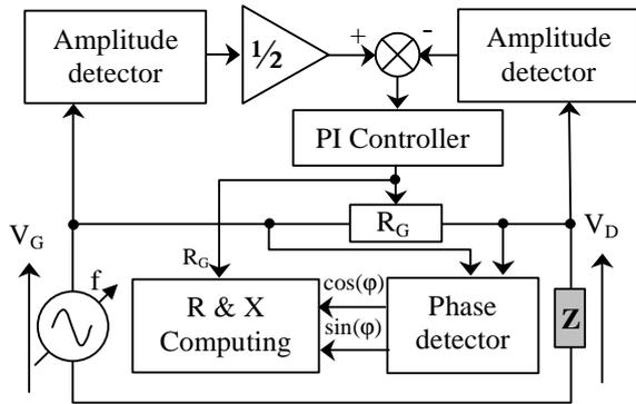
Figure 2. FVC method developed by Hamed and al.
