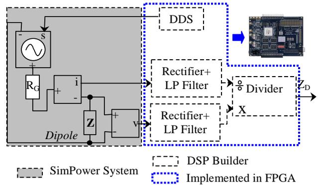
Figure 6. HIL scheme of the radiometric method
