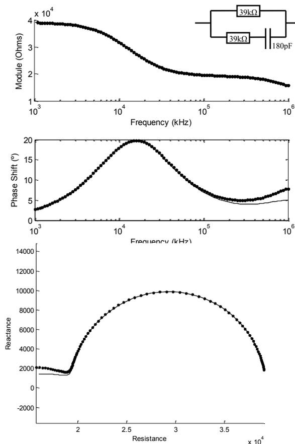
Figure 2. Bode and Cole-Cole diagram showing the reduction of cables capacitive effect by the application of the driven shield technique. The voltage mode excitation was used to analyze the circuit at the right top. The reduction is more noticeable at high frequencies where the capacitive effects have more influence.
