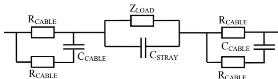
Figure 3. Equivalent electric circuit of all parasitic elements affecting impedance measurements of a load,  $Z_{LOAD}$ . The effect of the stray capacitances from cables,  $C_{CABLE}$ , is minimized by the driven shield. Other stray capacitance effect,  $C_{STRAY}$ , due primarily to the phase shift of amplifiers, can be minimized by software.
