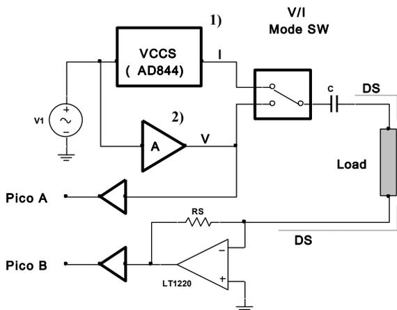
Figure 1. Schematic of the EIS system conditioning unit - 1) AC current source; 2) AC voltage source; 3) current/voltage sense.
