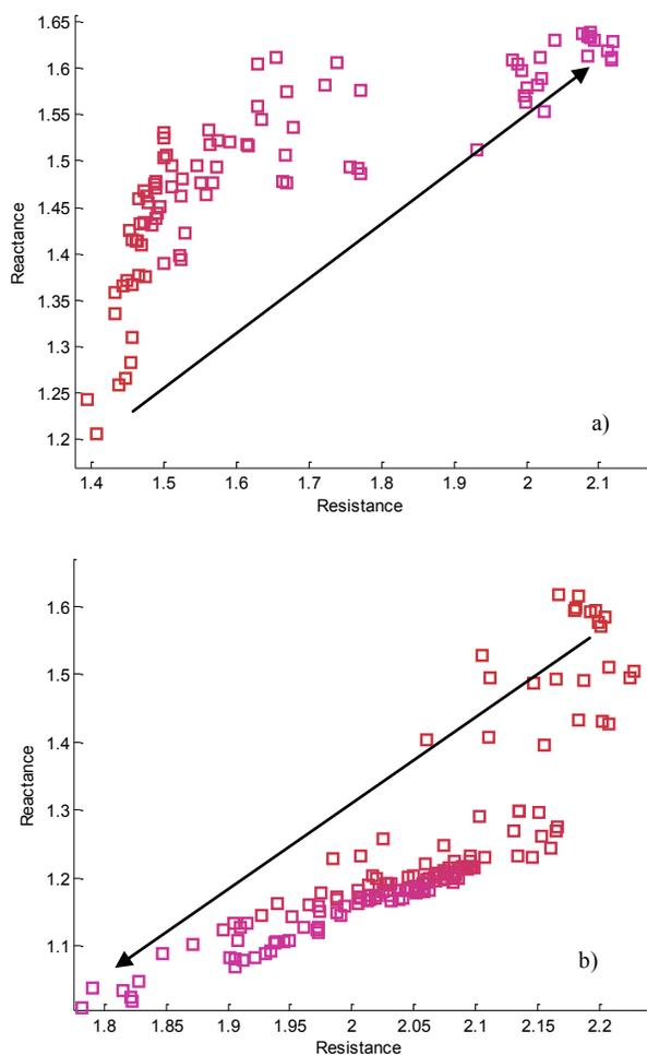
Figure 5. Evolution of the  $Z_1/Z_{50}$  ratio during the monitoring of a healthy chestnut tree a) while kept without watering and b) with regular watering. The arrows indicate the direction of the  $Z_1/Z_{50}$  ratio evolution.
