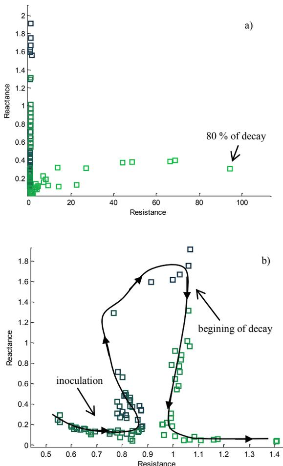
Figure 9. a) Evolution of the  $Z_1/Z_{50}$  during the monitoring time (8 weeks). b) Closer view from the  $Z_1/Z_{50}$  evolution, showing a hysteresis-like behaviour.
