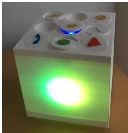
Figure 6. The RelaxedCare cube prototype that provides the overall wellbeing state of the assisted person via ambient lighting.
