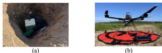
Figure 5. Data collection of buried sensor nodes by using a drone based on RSSI level: (a) Communicating sensor node buried at 30 cm depth before being covered by soil, (b) Drone used to collect the data.
