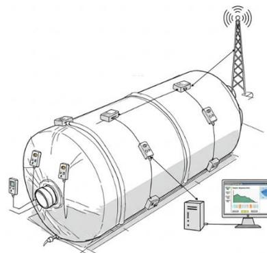
Figure 2. Ground communication network is formed by probes installed in the Silo, a hub (data concentrator) coupled to a ground station that transmits the signal to a database in the processing unit.
