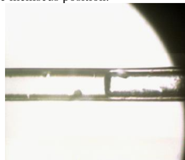
Figure 11. Video image of the meniscus in the capillary.
