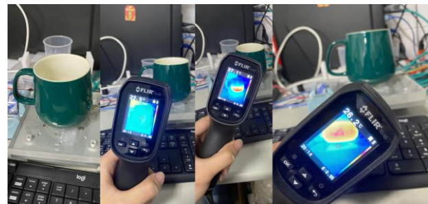
Figure 14. Infrared thermal imager temperature change
