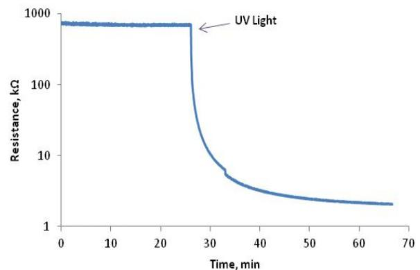
Figure 4. Resistance variation of the Co-doped SnO<sub>2</sub> sensing layer under the influence of UV irradiation at room temperature.
