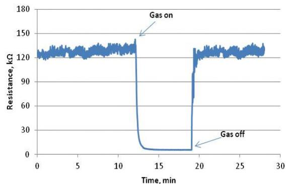
Figure 8. Resistance variation of the SnO<sub>2</sub><Co> sensor in the presence of 150 ppm ethanol vapors at 200 °C operating temperature in the dark.
