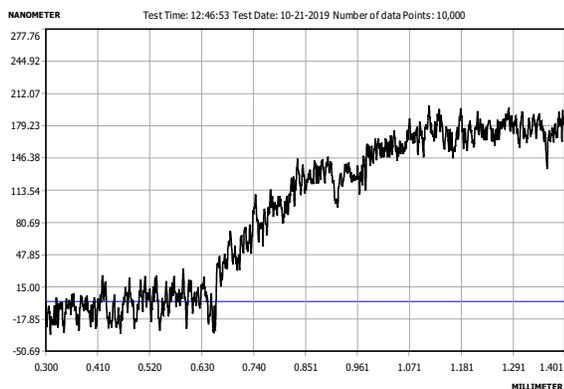
Figure 3. The thickness measurement result for the Co-doped SnO<sub>2</sub> film.
