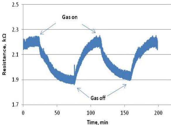
Figure 5. Resistance variation of the SnO<sub>2</sub><Co> sensor under the influence of UV irradiation at room temperature in the presence of 150 ppm ethanol vapors.
