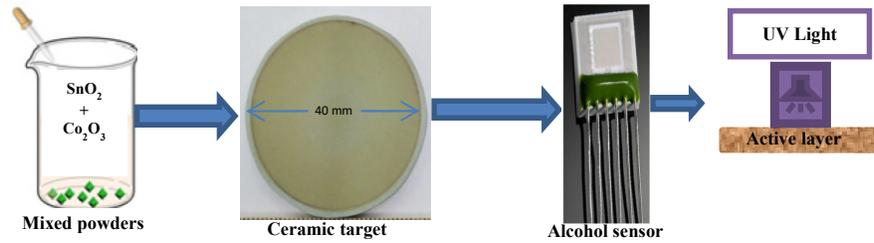
Figure 1. Schematic block diagram of the photo-assisted gas sensor fabrication.
