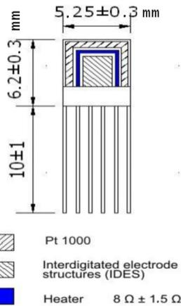
Figure 2. The schematic diagram of the Multi-Sensor-Platform.
