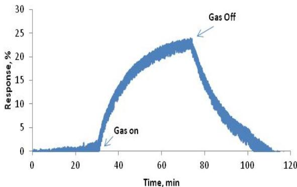
Figure 6. The SnO<sub>2</sub><Co> sensor response to 900 ppm of ethanol vapors under the influence of UV irradiation at room temperature.
