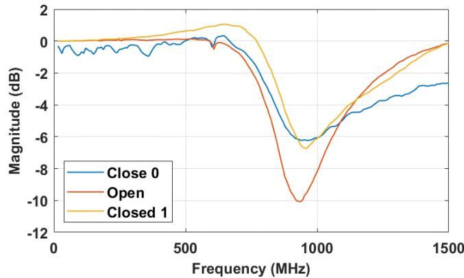
Figure 2.  $S_{11}$  magnitude for open and close states. Close 0 corresponds to the first attempt of closing the button, followed by Open when the button is released and finally Close 1 when the button is pressed again.
