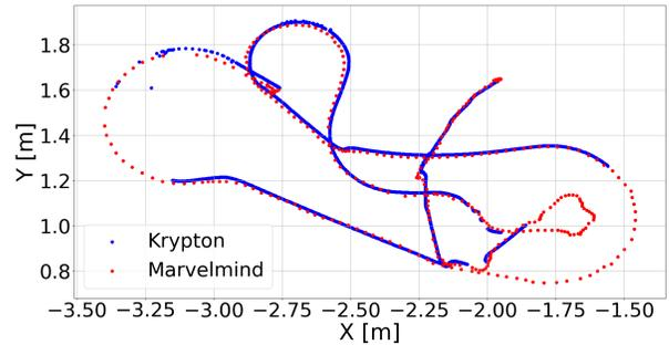
Figure 4. Marvelmind positioning results alongside Krypton CMM measurements.
