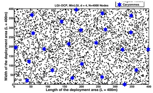
Figure 19. LQI-DCP: Average clusterhead locations, MinLQI criterion,  $N = 4000$  Nodes,  $R = 20m$ ,  $p = 0.75$ , multihop clustering  $d = 4$ .
