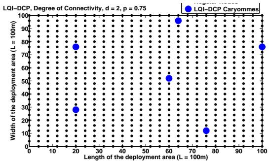
Figure 15. LQI-DCP: Average clusterhead locations, degree of connectivity criterion,  $R = 20m$ ,  $p = 0.75$ , multihop clusters  $d = 2$ .
