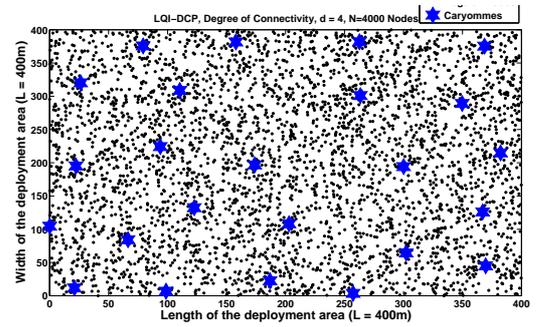
Figure 17. LQI-DCP: Average clusterhead locations, degree of connectivity criterion,  $N = 4000$  Nodes,  $R = 20m$ ,  $p = 0.75$ , multihop clusters  $d = 4$ .
