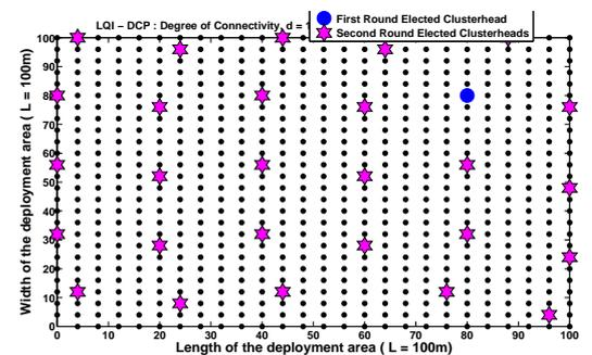
Figure 8. LQI-DCP: Average clusterhead locations, degree of connectivity criterion,  $d = 1$
