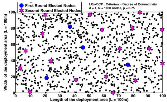
Figure 14. LQI-DCP: Average clusterhead locations, degree of connectivity criterion,  $d = 1$ ,  $p = 0.75$
