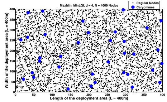
Figure 18. MaxMin: Average clusterhead locations, MinLQI criterion,  $N = 4000$  Nodes,  $R = 20m$ ,  $p = 0$ , multihop clustering  $d = 4$ .
