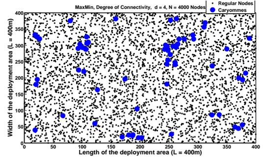
Figure 16. MaxMin: Average clusterhead locations, degree of connectivity criterion,  $N = 4000$  Nodes,  $R = 20m$ ,  $p = 0$ , multihop clusters  $d = 4$ .
