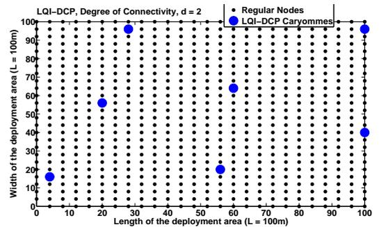
Figure 9. LQI-DCP: Average clusterhead locations, degree of connectivity criterion,  $d = 2$
