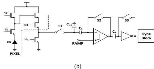
Figure 1. Principle of a Conventional CMOS Image Sensor (CIS)
