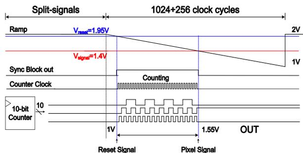
Figure 4. Timing Diagram of the Proposed Intelligent One-ramp CDS
