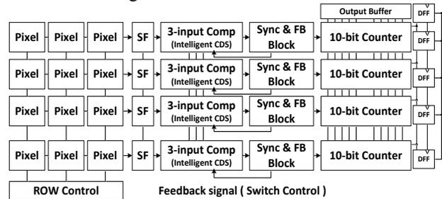
Figure 5. Block Diagram of the CIS with an Intelligent CDS
