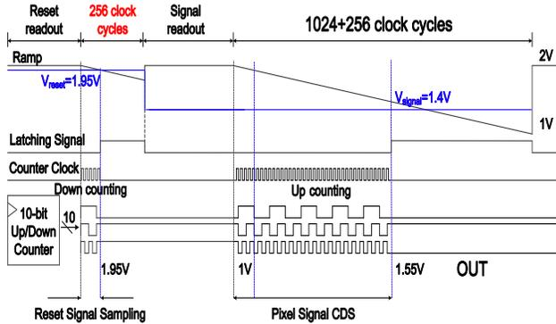
Figure 2. Timing Diagram of a Conventional Two-ramps Digital CDS
