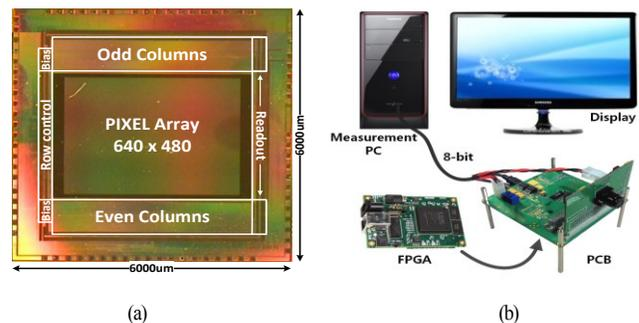
Figure 6. Chip Photo and Measurement (a)Chip Microphotograph of the CIS with Samsung 0.13μm CIS (b) Configuration of the Measurement Systems
