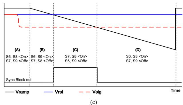
Figure 3. Principle of the Proposed CDS
