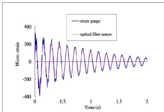
Figure 4. Dynamic strain of a cantilever beam impacted by a hammer
