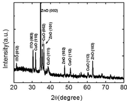
Figure 2. Typical X-ray diffraction pattern of the CuO thin film/ZnO nanorods heterostructure fabricated on an ITO-coated glass substrate.
