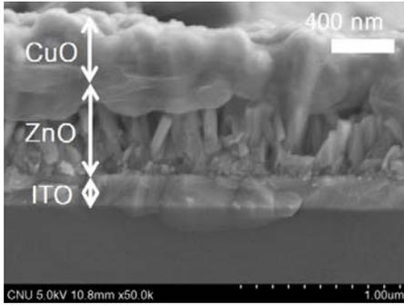
Figure 1. Cross-sectional SEM image of the CuO thin film/ZnO nanorods heterostructure fabricated on an ITO-coated glass substrate.
