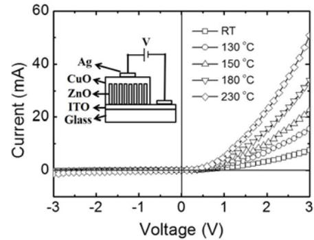
Figure 3. Current–voltage ( $I$ – $V$ ) characteristic curves of the CuO thin film/ZnO nanorods heterostructure in dry air at several temperatures. The inset shows a schematic circuit of the oxide p–n heterojunction device.
