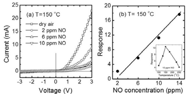
Figure 4. (a) Current–voltage ( $I$ – $V$ ) characteristic curves of the CuO thin film/ZnO nanorods heterojunction diode structure for several NO gas concentration in dry air at  $150 \text{ }^\circ\text{C}$ . (b) Variation of the sensitivity as a function of the NO gas concentration in dry air.
