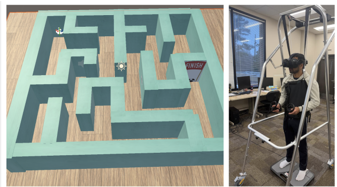
Figure 2. a) Top-down view of the virtual maze environment. b) Participants navigating the virtual maze while standing on the balance board and wearing a harness for safety.
