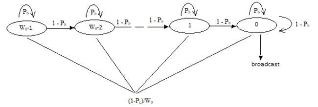
Figure 2. Back-off Process via Markov Chain Model
