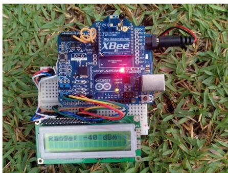
Figure 5. Receiving device standing on the ground, during first measurement.
