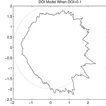
Figure 4. Irregularity coefficient in the radio coverage.
