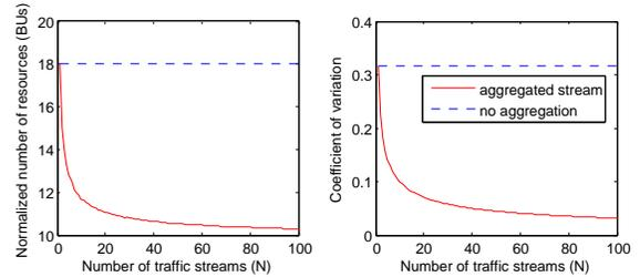
Figure 2. Analysis of multiplexing gain with aggregation.
