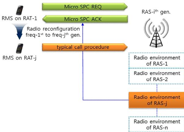
Figure 6. Operation of handover by exchanging adjacent channel information
