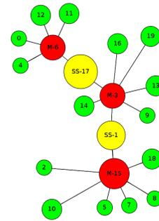
Figure 1. Common Scatternet of 20 devices found by simulation
