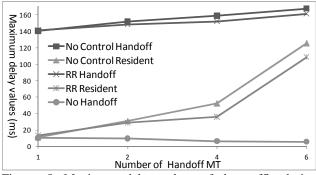
Figure. 5. Maximum delay values of the traffic during handoff affection period
