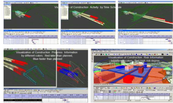
Figure 2. Application of BIM object for construction project
