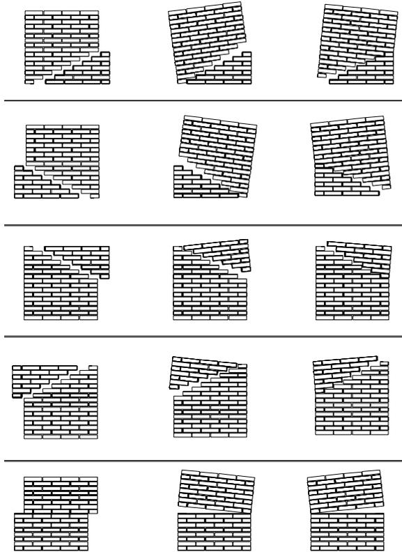
Figure 1. Possible mechanisms that a single FE represents.
