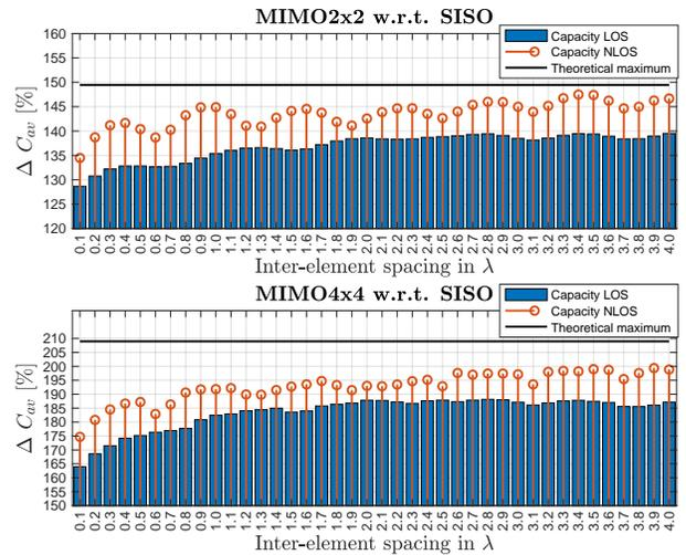
Figure 4. V2I channel capacity for different inter-element spacing for MIMO 2x2 and MIMO 4x4 with respect to the SISO channel capacity in percent and a fixed SNR of 10 dB.
