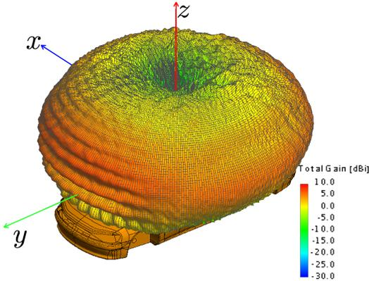
(b) Radiation pattern of a monopole mounted on the car rooftop.
