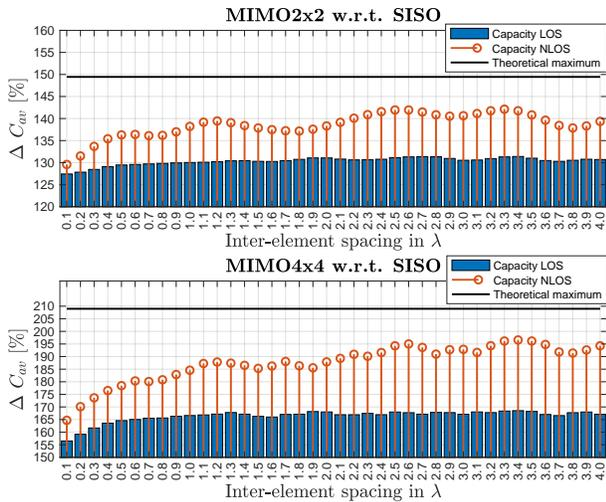
Figure 5. V2V channel capacity for different inter-element spacing for MIMO 2x2 and MIMO 4x4 with respect to the SISO channel capacity in percent and a fixed SNR of 10 dB.
