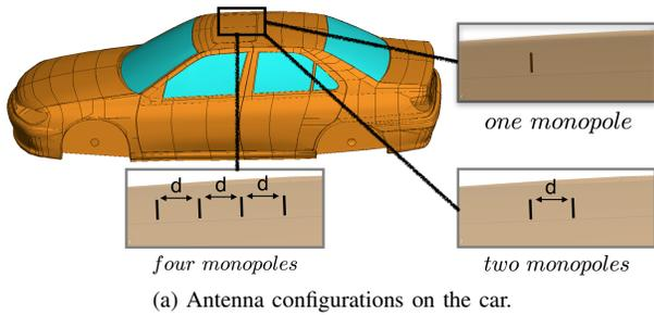
(a) Antenna configurations on the car.
