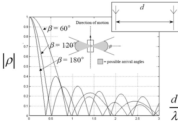
Figure 1. Correlation for two dipoles with changing inter-element spacing and three distinct angle of arrival [7].
