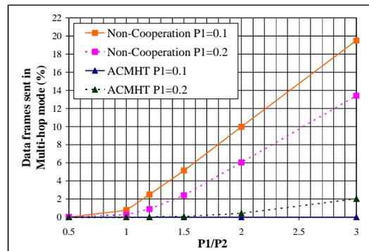
Figure 11. The percentage of data frames sent in multi-hop mode in scenario 2 of the 5-terminal networks.
