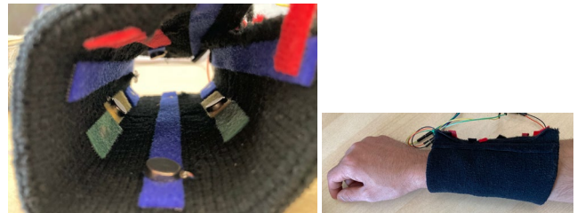
Figure 1. (a) Sleeve embedded with the four motors in the spaced-ring arrangement. (b) Sleeve worn by one of the participants.
