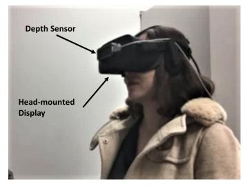
Figure 7. The remote user's wearable device: a head-mounted display with a depth sensor attached to its front side
