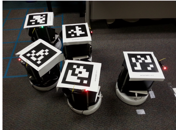
Figure 2. The TurtleBot swarm always has one leader. The leader may be an Active Leader (green LED, shown) or an Inactive Leader (blue LED).
