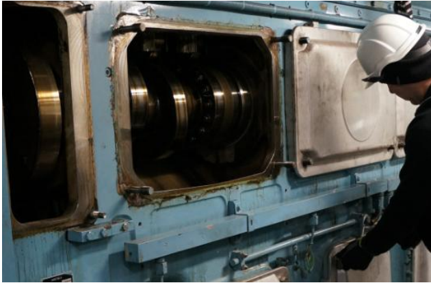
Figure 1. Checking the condition and function of an engine's overhaul hatch.
