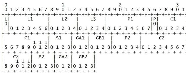
Figure 1. Example of G.729 and G.729A bit packing.
