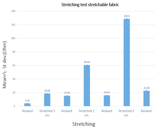
Figure 7. Stretching test results for stretchable fabric
