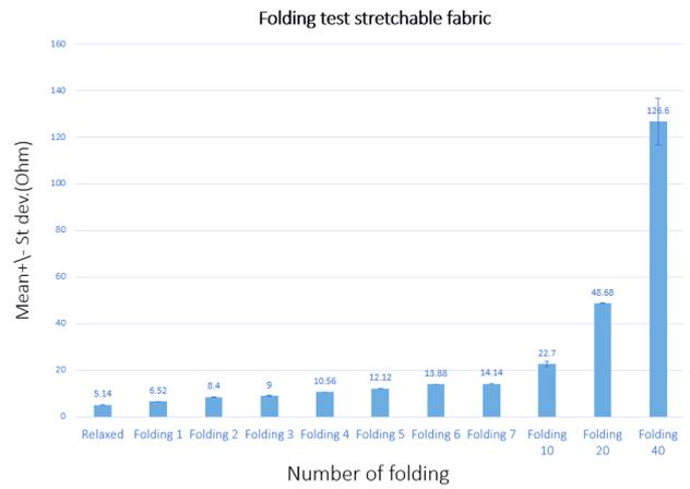
Figure 9. Folding test results for stretchable fabric
