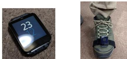
(a) WD: SmartWatch 3, Sony (b) WD mounted on foot
