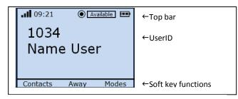
Figure 15. Ascom 9d24 prototype main screen
