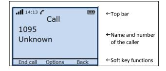
Figure 20. Ascom 9d24 prototype Incoming call (name & number)
