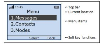
Figure 16. Ascom 9d24 prototype main menu
