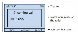
Figure 19. Ascom 9d24 prototype Incoming call (number)
