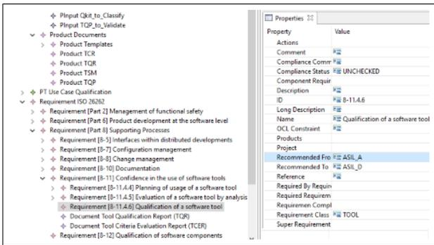
Figure 6. Expanded nodes for requirements in the TOPWATER tool.
