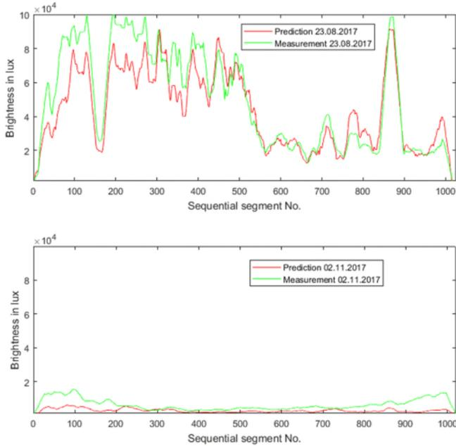
Figure 8. Results of the solar radiation prediction
