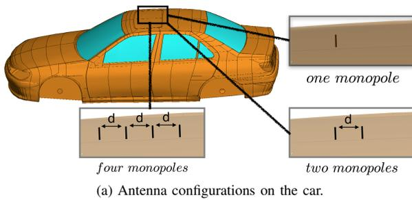
(a) Antenna configurations on the car.
