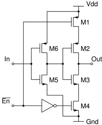
Figure 4. Standard design of a tristate buffer
