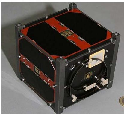
Figure 4. An example of a 1U cubesat [22].
