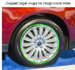
Figure 17. Successful Hough ellipse match to rear wheel (match highlighted in green).
