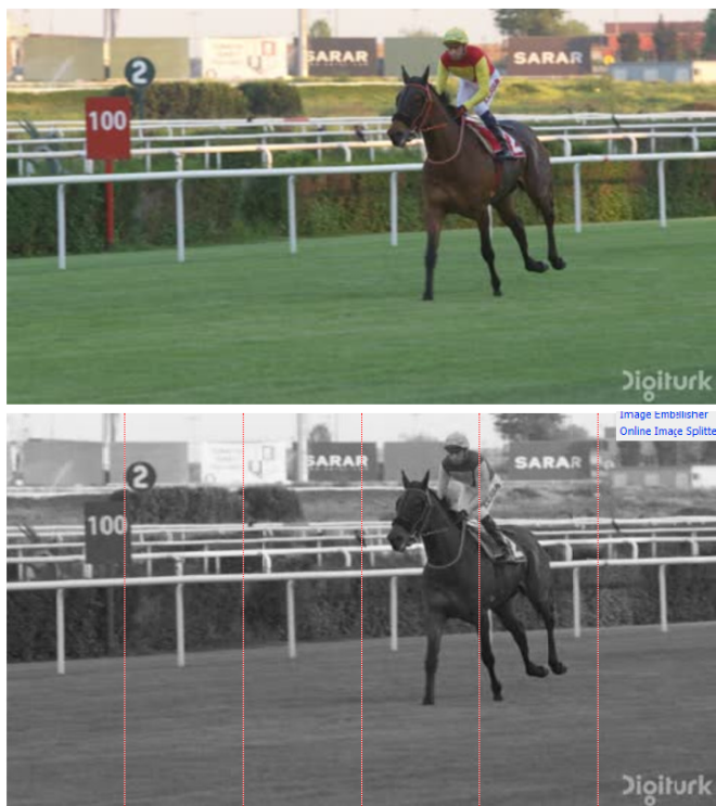
Figure 1. Example of a full-FoV UHD video frame (top) and its corresponding partitioning into 6 FoVs (bottom).
