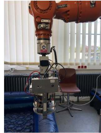
Figure 1b. Sensors mounted on the miniature drill-head and further mounted on the KUKA robotic arm
