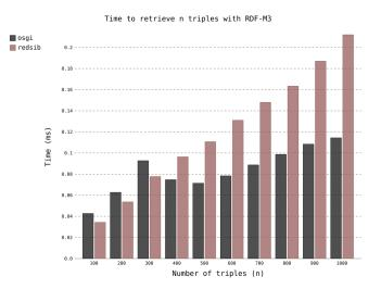
Fig. 5. The Query test performed on RedSIB and OSGi SIB to retrieve the entire RDF store content using the RDF-M3 query formalism
