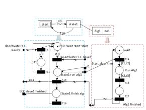
Figure 6. GR-TNCES model of ECC<sub>slave1</sub>.
