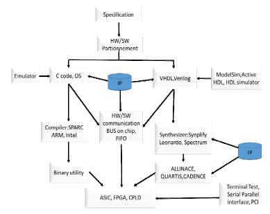
Figure.1. Flow of system design of SoC
