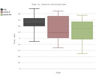
Fig. 7. The Subscription Test performed on RedSIB (with options --ram and --ram-hash) and OSGi SIB
