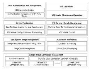
Figure 3. Functional blocks of multiple Clouds based VDI management
