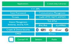
Figure 3. MBED stack from the ARM company
