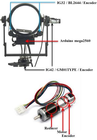
Figure 7. The composition of the proposed hardware to be attached to the camera
