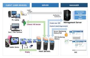
Figure 1. General VDI service architecture in single Cloud
