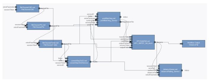
Figure 2. The graphical user interface of WFE, where dotted lines represent flow of services, while solid lines connect parameters from outputs to inputs.
