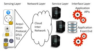
Figure 1. An IoT service-oriented architecture (SoA), based on four layers
