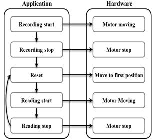
Figure 3. The work flow of the proposed application and hardware attached to the camera
