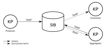
Fig. 1. The architecture of the Smart-M3 interoperability platform
