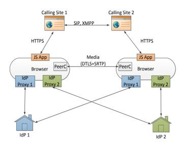
Fig. 1. WebRTC Communication Model
