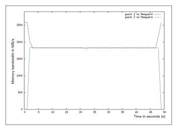
Figure 7. Memory bandwidth degradation between two guests
