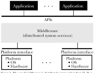
Figure 1. The set of middleware in distributed system, taken from [3..7], p. 89
