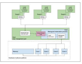
Figure 4. Proposed extensions to Memguard's architecture
