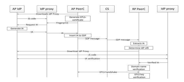
Fig. 2. End-to-End Authentication Flow Diagram
