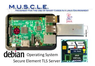
Figure 8. TLS Server satck embeded in secure element, in a Raspberry Pi environnment.
