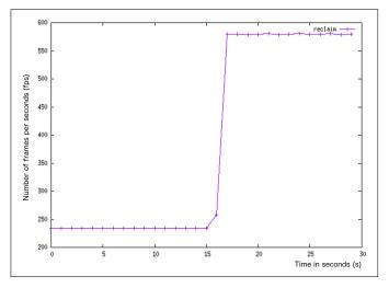
Figure 2. Memory bandwidth reclaim feature
