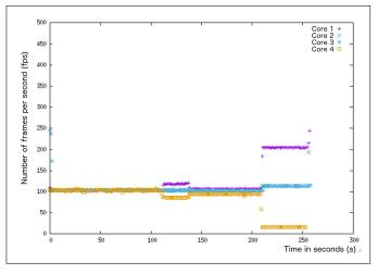
Figure 1. Memory bandwidth reservation on different cores
