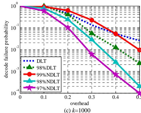
Figure 4. Overhead and decoding failure probability of distributed LT and new distributed LT of recovering 99%, 98%, 97% of original information.
