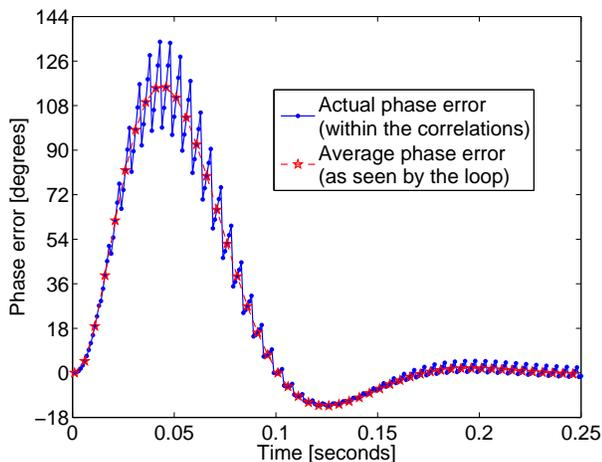
Figure 2. Phase estimation error during a step of 20g.
