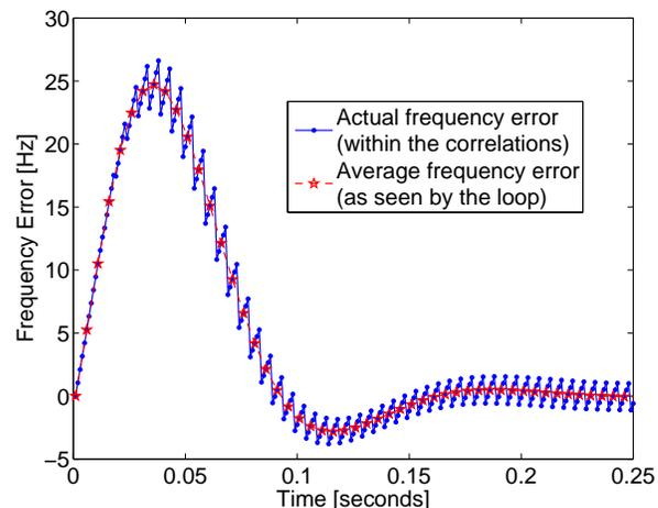
Figure 3. Frequency estimation error during a step of 20g.
