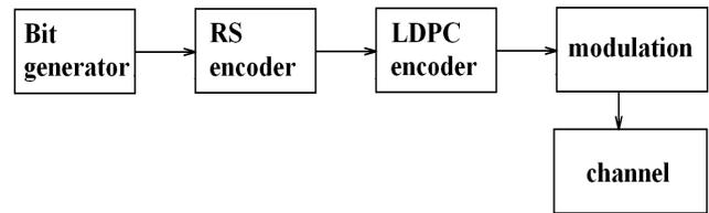
Figure 3. Simplified block scheme of new transmitter model
