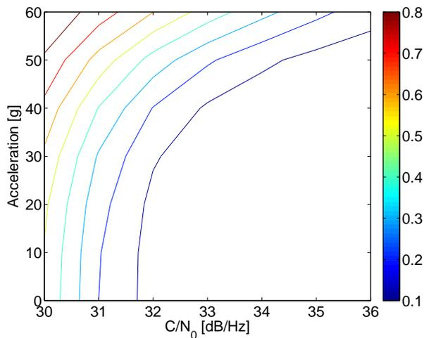
Figure 6. POP of bit-asynchronous loop and its tracking threshold.
