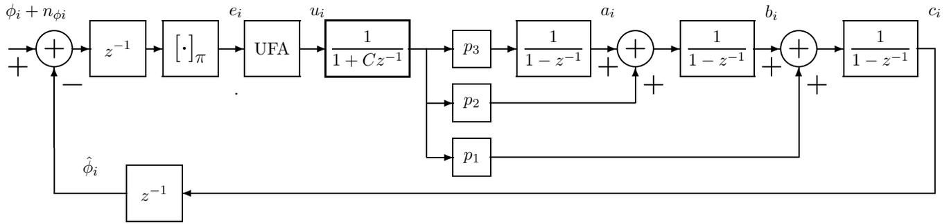
Figure 1. Block diagram of the UFA-PLL model.
