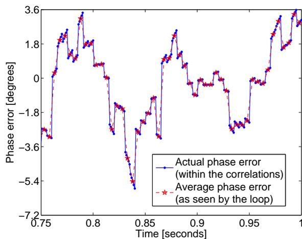
Figure 4. Phase estimation error with  $C/N_0 = 48$  dB/Hz.
