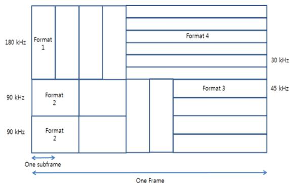
Figure 2. Uplink PUSCH channel structure for narrowband transmission.
