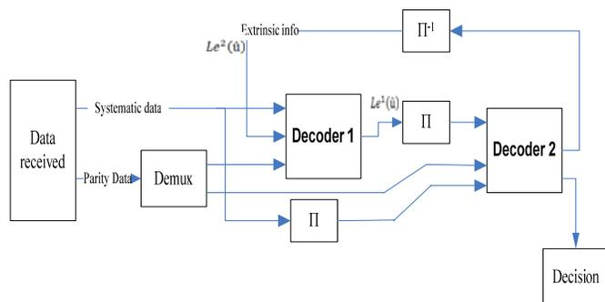
Figure 2. Basic structure of an iterative turbo decoder
