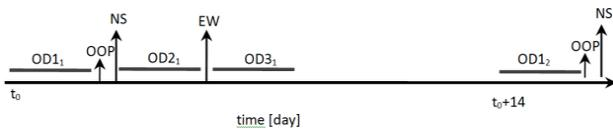
Figure 1. Station Keeping Principle of TURKSAT 3A
