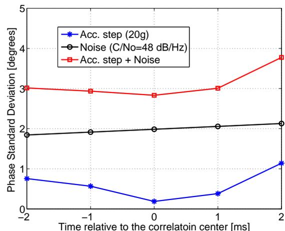
Figure 5. Phase estimation error within the correlation interval.
