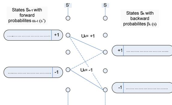
Figure 3. Trellis structure of systematic convolutional codes
