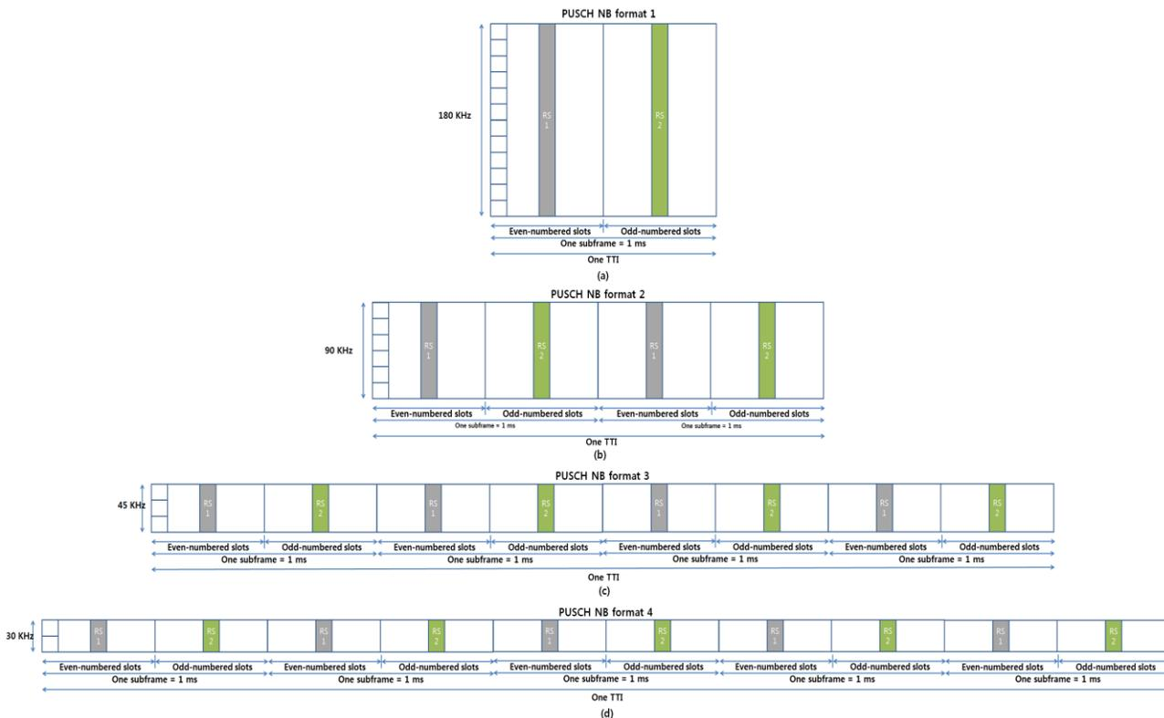
Figure 1. Uplink PUSCH channel structure for narrowband transmission.
