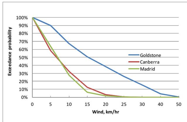
Figure 2. Exceedance probability distribution of wind speed at three tracking complexes.
