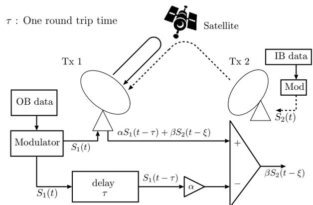
Fig. 2. Concept of interference canceller for superposed transmission.
