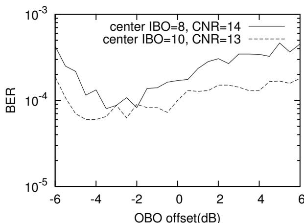
Fig. 9. BER difference when rain attenuation level changes.
