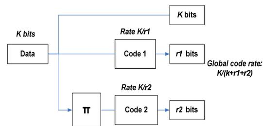
Figure 1. Basic structure of the turbo encoder
