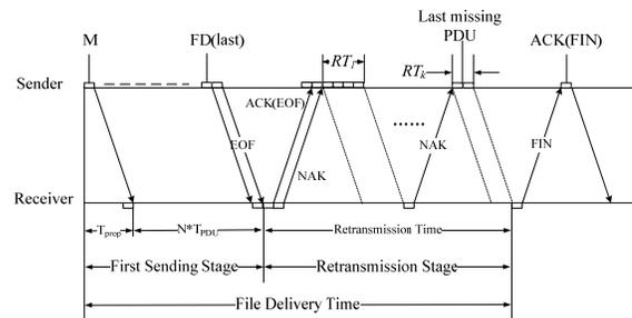
Figure 1. Delay time diagram of  $K$ -retransmission-based deferred NAK.
