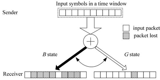
Figure 1. Two error state AWGN channel Gilbert-Elliot model
