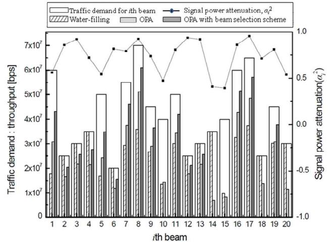
Figure 2. The comparison of throughput of  $i$ th beam for water-filling, OPA scheme and OPA scheme with selective beam allocation
