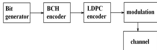
Figure 1. Simplified DVB-S2 transmitter model.
