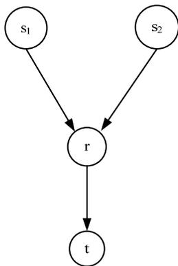
Figure 1. A two-source single-sink relay network
