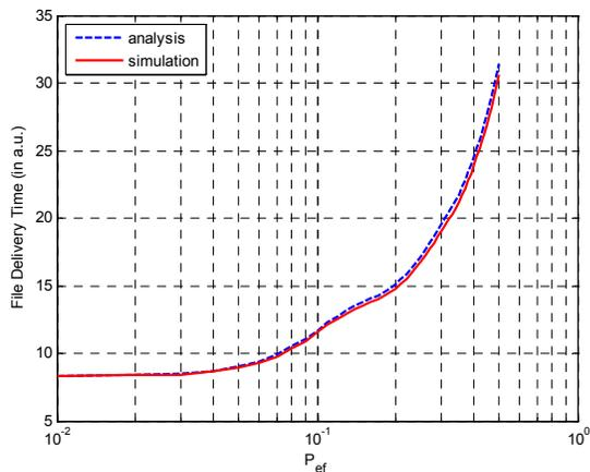
Figure 4. DR deferred NAK: analytic and simulation results. File size = 1MB, transmission rate = 20kb/s, and one way propagation delay = 2.5 a.u.
