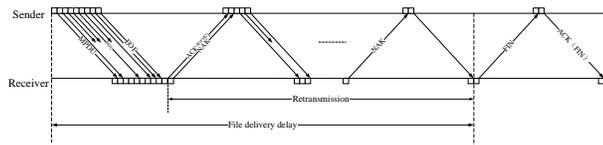
Figure 1. Process of CFDP deferred NAK mode transmission
