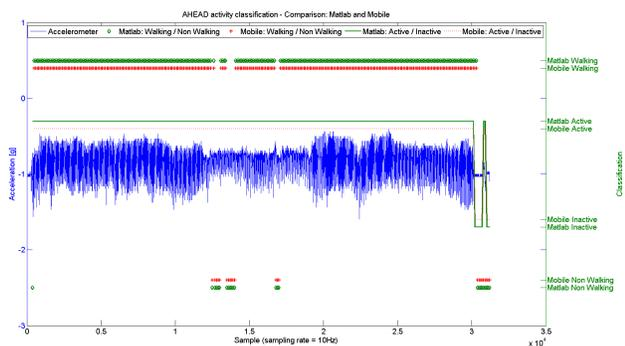
Figure 4. Illustration of AHEAD classification (walking/non walking, active/inactive) durind a walking sequence
