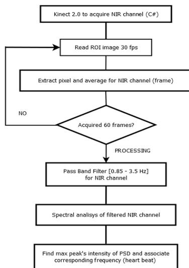
Figure 1. Block diagram real-time processing NIR channel.
