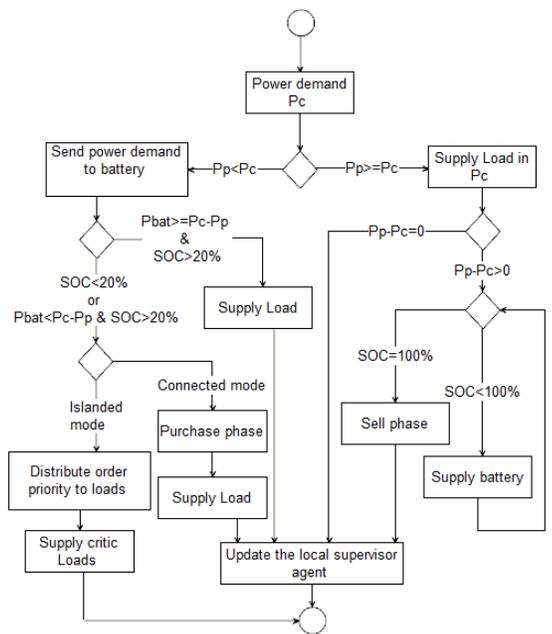
Figure 4. Proposed management algorithm for microgrid operation
