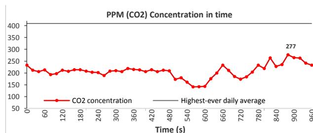
Figure 8. CO<sub>2</sub> values [PPM] collected with MQ 135 gas sensor from a heavy traffic boulevard from Sibiu
