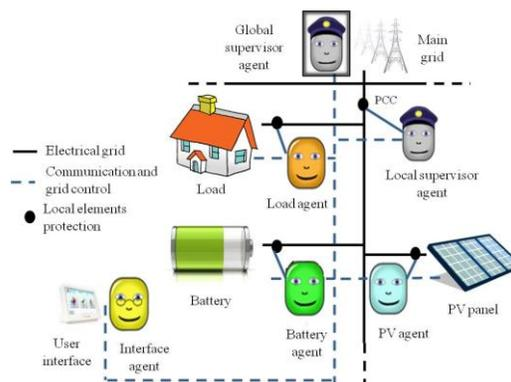
Figure 2. MAS for the proposed Microgrid management approach
