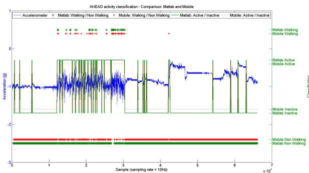
Figure 3. Illustration of AHEAD classification (walking/non walking, active/inactive) durind daily life activities
