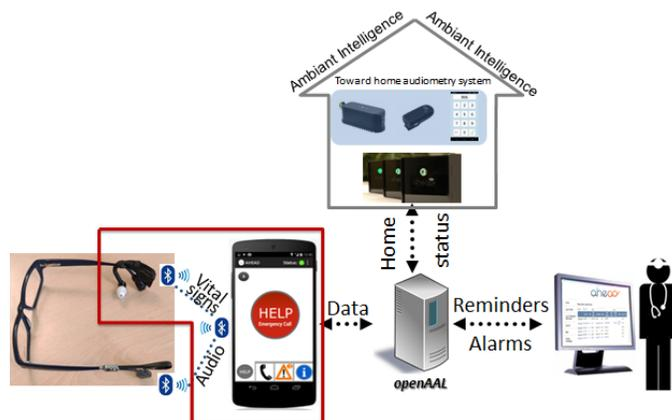
Figure 1. Overall AHEAD components
