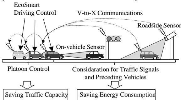
Figure 1. Concept of Proposed EcoSmart Driving Control.
