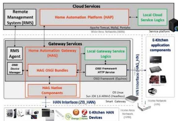
Figure 6. Hardware architecture.
