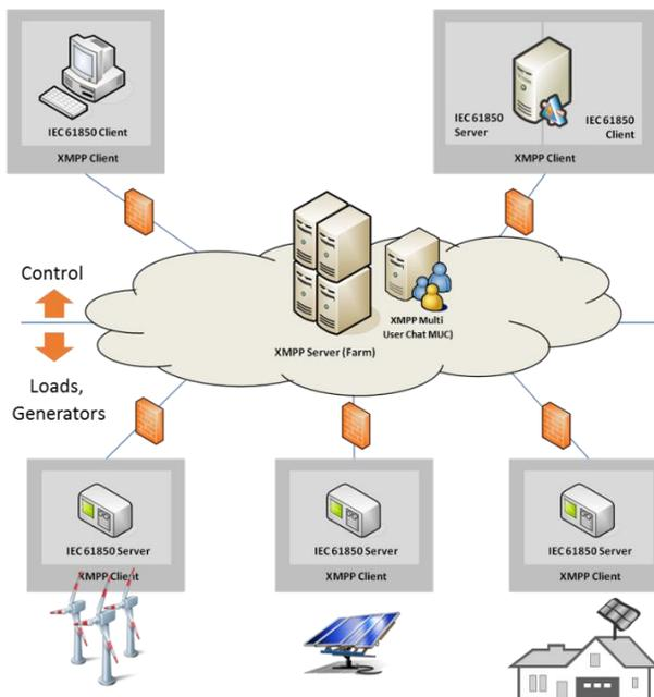
Figure 1. DER Integration based on IEC 61850 over XMPP
