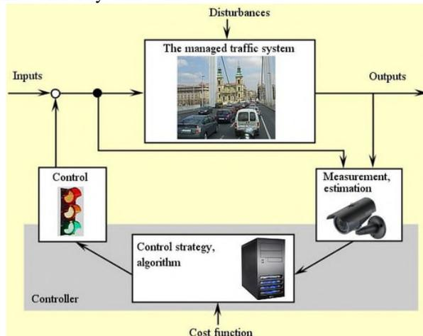
Figure 2. The adaptive urban traffic control system works.
