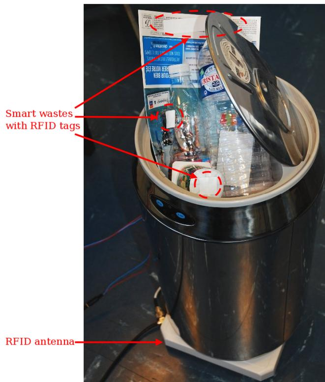
Figure 6. An individual bin using the RFID technology.
