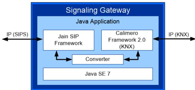
Figure 3. Connection interfaces of the Signaling Gateway
