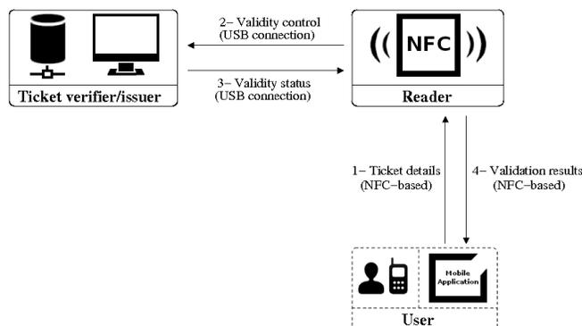
Figure 7. Architecture of the inverse reader model
