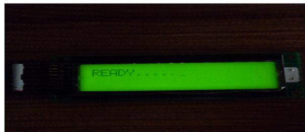
Figure 8. Display after initializing
