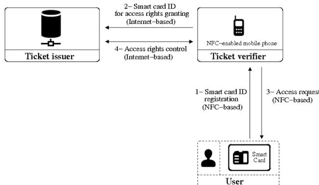
Figure 6. Architecture of the leeches smart card model
