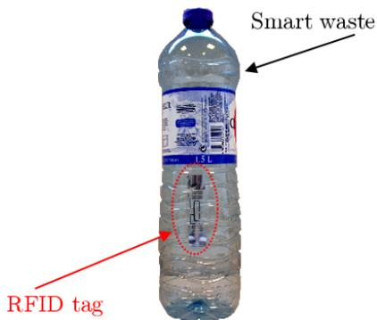
Figure 2. An example of a smart waste.
