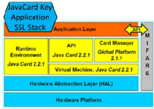
Figure 4. Illustration of a dual interfaces application
