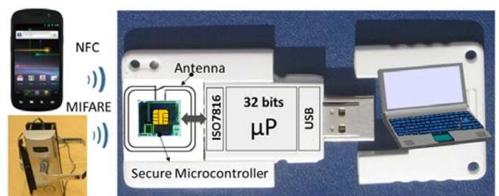
Figure 2. Triple Interface Secure Token (TIST) hardware architecture
