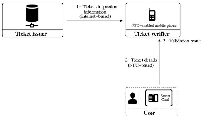
Figure 5. Architecture of the smart card-based model
