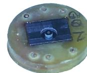
Figure 4. MEMs force sensor connected and mounted in PCB
