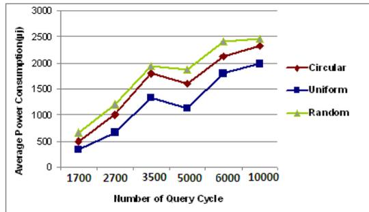
Figure 9. Average Power Consumption for different Query Cycle.
