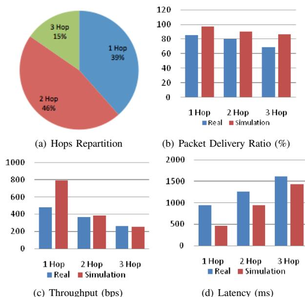
Figure 5. Performances of real and simulated PLC network
