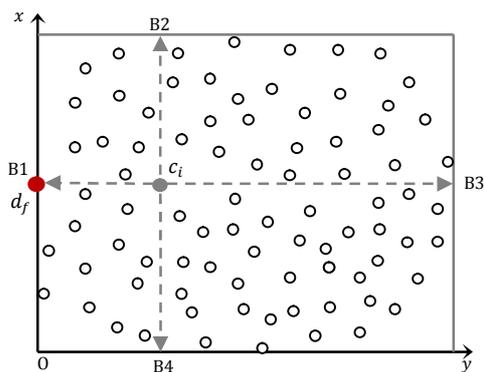
Figure 4. Fictitious destination  $d_f$  for the NBD algorithm.
