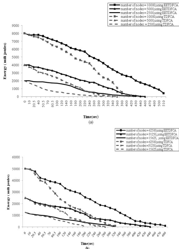
Figure 1. Remaining energy in the network (a) in first scenario (100\*100) (b) in second scenario (250\*250) EETDFCA in comparison with TDFCA
