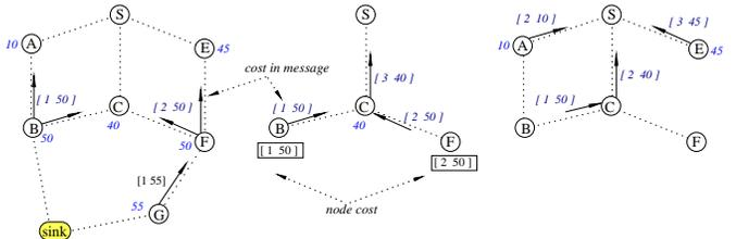
Fig. 1. Cost establishment process: a) Nodes  $G$ ,  $B$ , and  $F$  send their cost; b)  $C$  receives first the packet from  $F$  and it broadcasts the cost  $[3, 40]$ ; c)  $C$  receives a smaller cost from  $B$  and broadcasts again the cost  $[2, 40]$ . Nodes  $A$  and  $E$  send their cost. The source  $S$  knows three paths (along nodes  $A$ ,  $C$ ,  $E$ ) and selects the path with the smaller cost (along  $C$ ).
