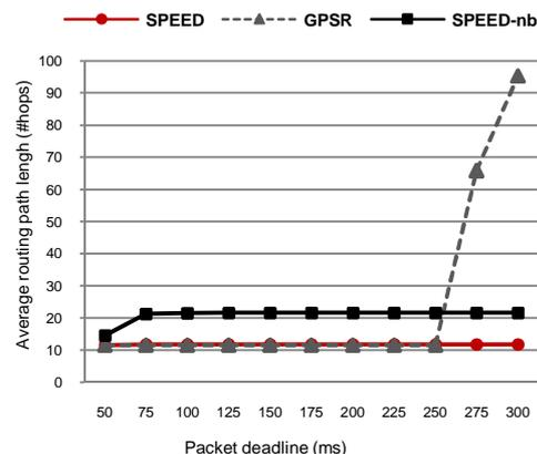
Figure 10. Average routing path length of delivered packets.
