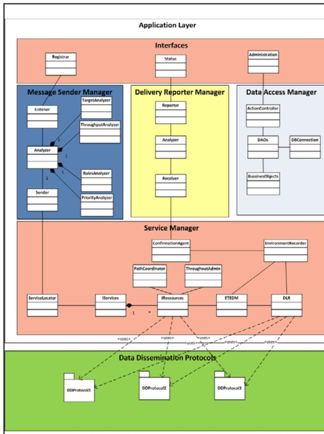
Figure 5. Class diagram of the reference architecture.
