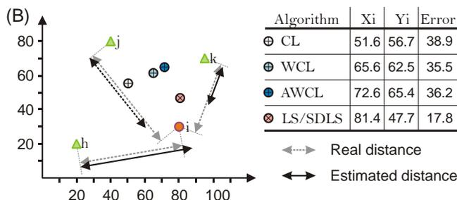
Figure 1. Example Localization (A) Example setup with erroneous distance estimations, (B) Visualization and results. All values in meters.
