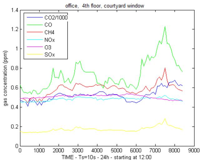
Figure 5. Gas concentration (ppm) of the acquisition realized within a 4th floor office of the hospital with a courtyards window.
