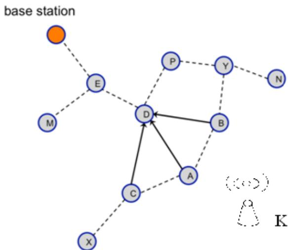
Figure 1: Wireless sensor network communication topology.
