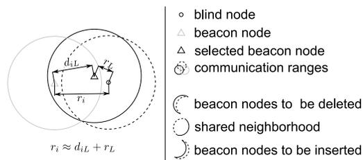
Figure 3. Approximation of a distance between blind node and inaccessible beacon node  $i$  by means of the linearizing beacon node  $L$
