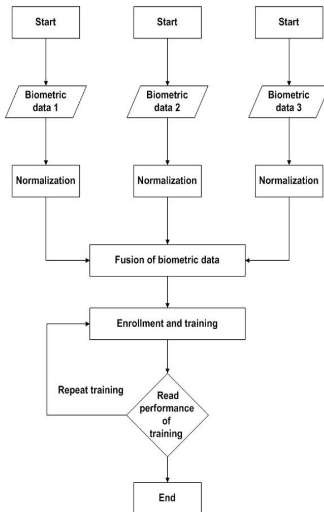
Figure 1. Flowchart showing the design of the system
