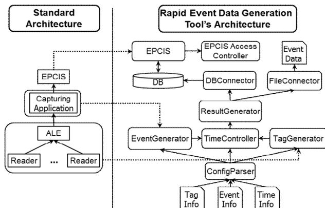
Figure 5. Architecture of the test data generation tool
