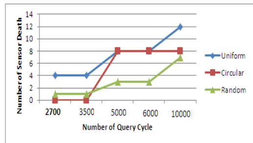
Figure 8. Rate of Sensor death for three Sensor Placement Strategies.
