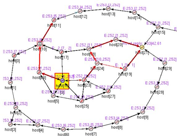
Fig. 3. Data forwarding on the path 26-10-11-12-...(lightblue arrow).
