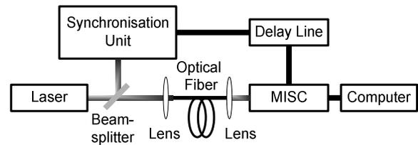
Figure 6. Experimental setup for repetitive pulses observation
