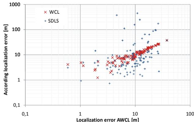
Figure 7. Correlation between sorted localization errors of SDLS-measurements and according localization errors of AWCL
