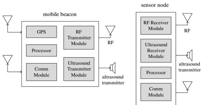
Fig. 1. Block diagram of the mobile beacon and sensor node.
