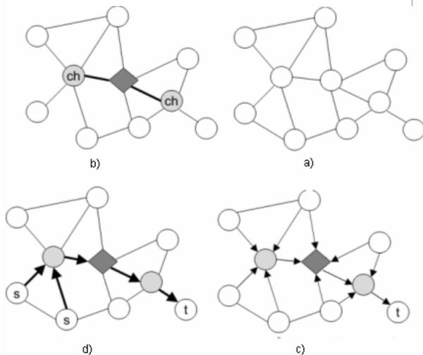
Figure 3. structure of clustered directed diffusion (Gray circles are head of groups and diamonds are the gates)
