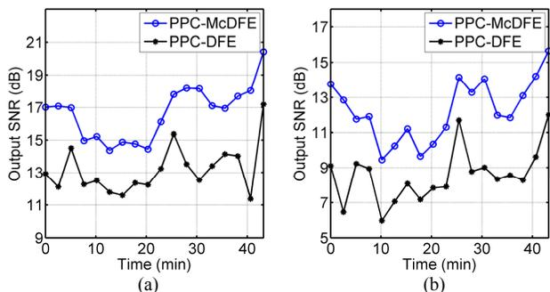
Figure 8. The performance in terms of output SNR. (a) BPSK. (b) QPSK.
