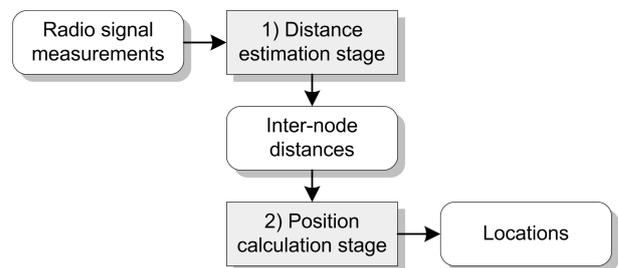
Figure 1. The scheme of localization process
