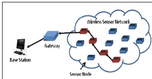
Figure 1. Example of a Wireless Sensor Network.
