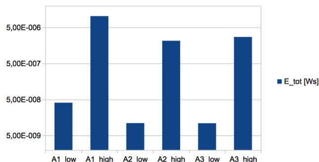
Figure 6. Energy usage for different WSN node architectures for a piezo electric based ultrasound pulse echo WSN node.
