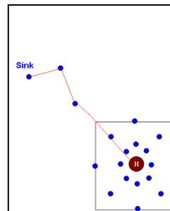
Figure 3. Circular Clustered-Distribution of 16 sensor nodes.
