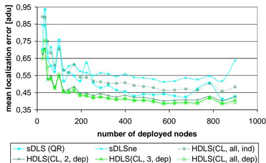
Figure 15. Mean localization error of CL based HDLS with dependent distance estimation
