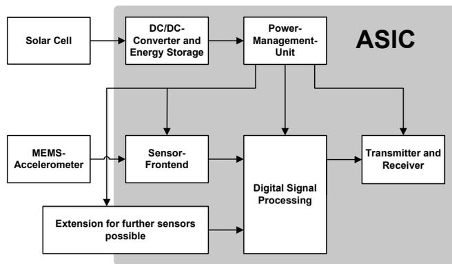
Fig. 6. Block diagram sensor node.
