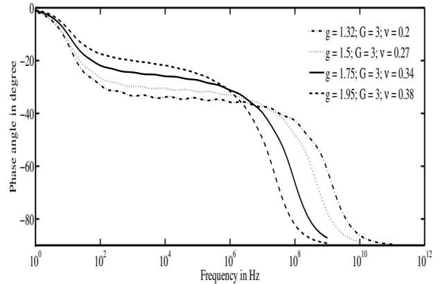
Figure 9. Simulation results showing change in ' $\alpha$ ' with change in ratios ' $g$ ' and ' $G$ '
