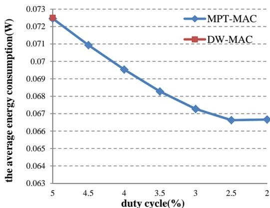
Fig. 15: Average EDL of MPT-MAC with different duty cycle
