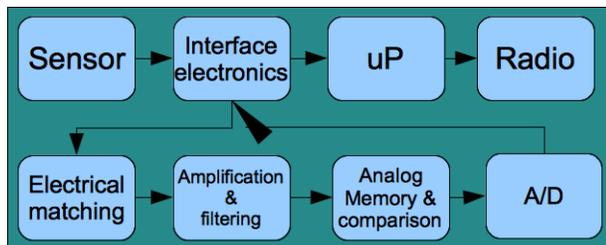
Figure 3. WSN node architecture, A3, with external analog memory and comparison logic before the A/D conversion.
