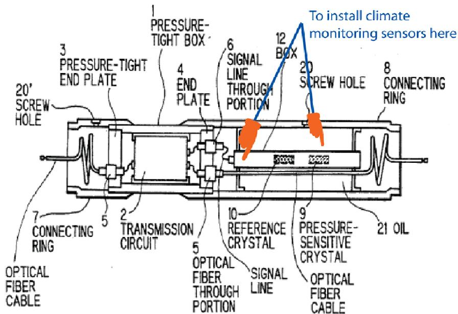
Figure 3. Cable and repeaters are being laid down in the ocean (upper panel), a view of open Alcatel-Lucent repeater (middle panel) and the diagram of a submarine cable repeater (lower panel). Climate monitoring sensors could be integrated into the equipment and the measured signals transmitted back to a shore station via the repeater's transmission device.
