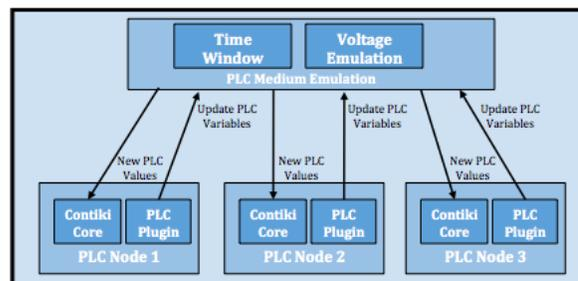
Figure 1. A simulated PLC environment in COOJA
