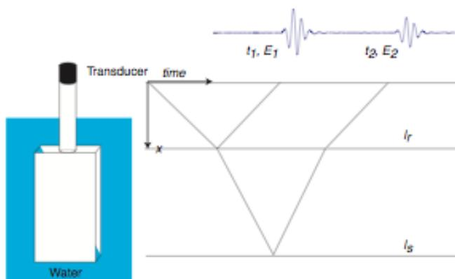
Figure 5. Ultrasound pulse echo measurement with associated acoustic signals
