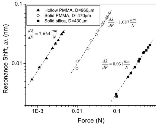
Figure 11. Force versus Resonance results for different spheres [16].
