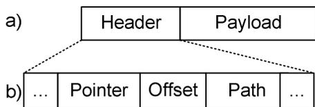
Figure 2. a) Packet generated by BS, b) Header of the packet
