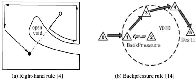
Figure 2. Classes of techniques handling open voids.
