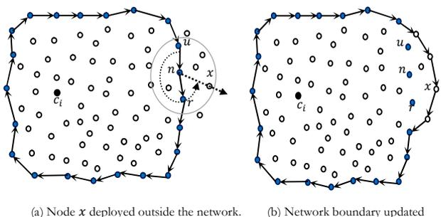
Figure 7. Network boundary updating after a node deployment.
