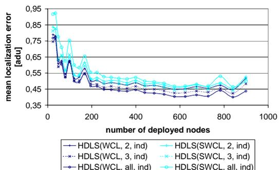
Figure 9. Mean localization error of HDLS based on WCL and SWCL with independent distance estimation
