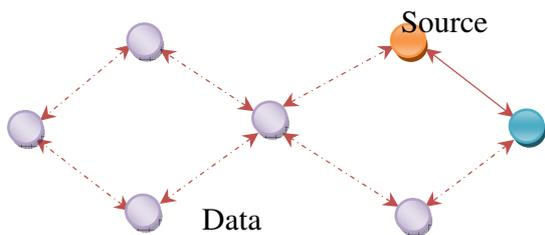
Figure 1. operation of diffusion in forwarding the discovery data
