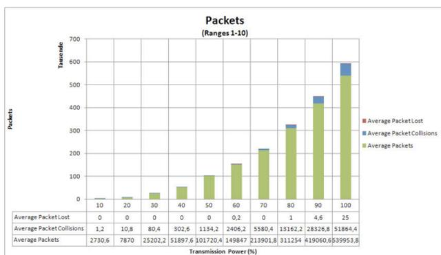
Figure 5. Traffic load in relation to signal strength
