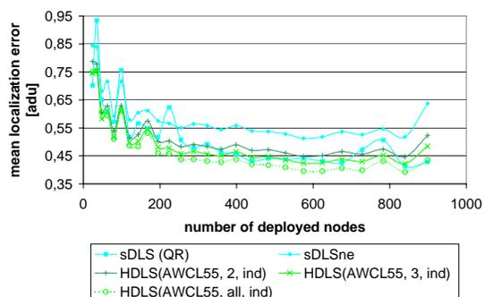
Figure 10. Mean localization error of AWCL based HDLS with independent distance estimation
