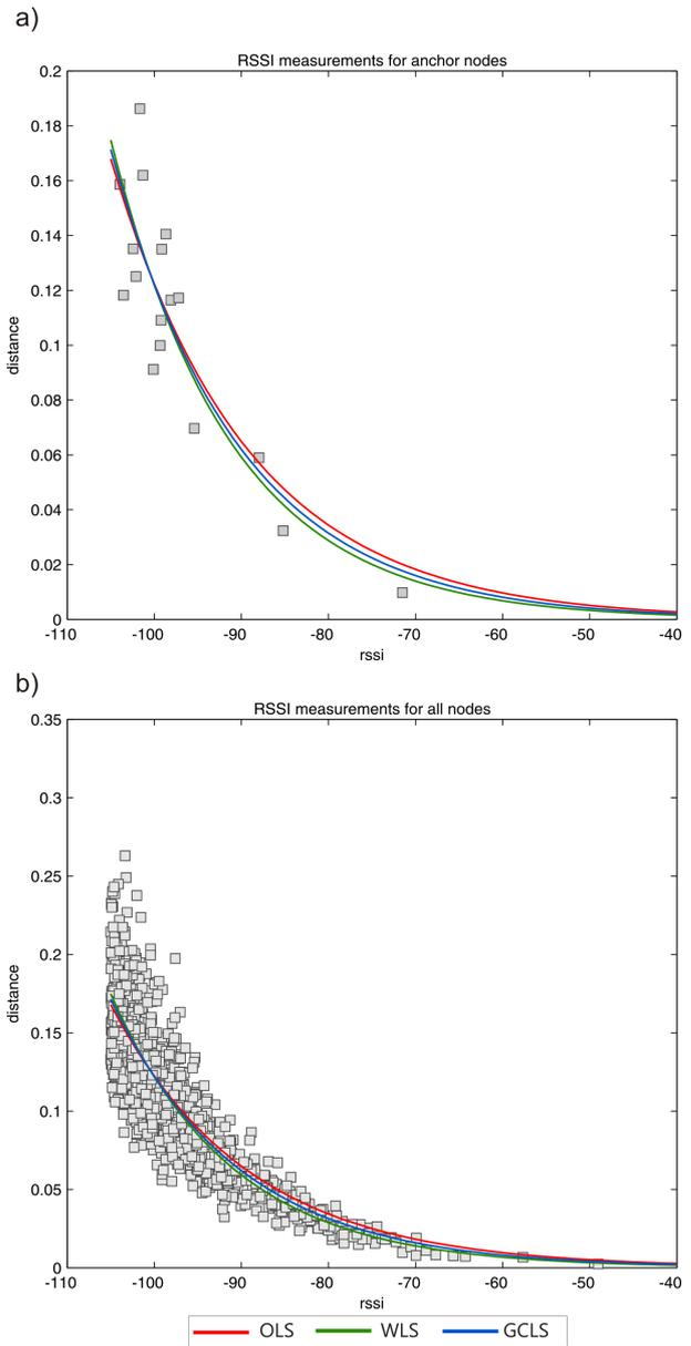
Figure 5. Distance as a function of RSSI measurements.
