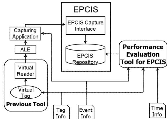
Figure 9. Test System Environment
