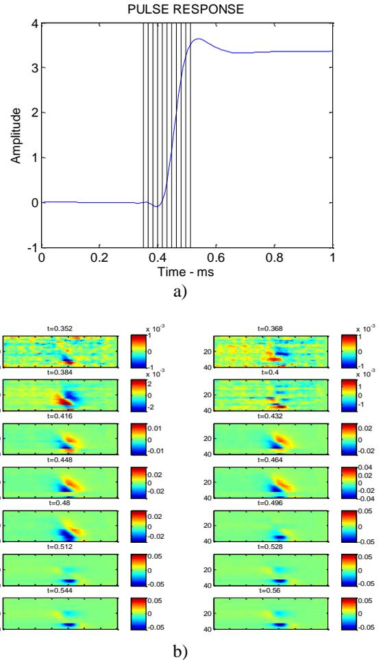
Fig. 6: a) Pulse response with time slots marked, b) Result of imaging the transient response from the hunting knife.
