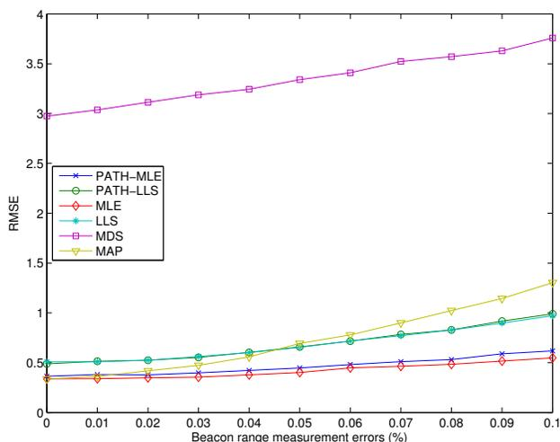
Fig. 5. The RMSE of location estimates versus  $\kappa$ : C-shape grid network.
