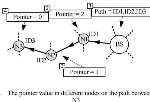
Figure 3. The pointer value in different nodes on the path between BS and N3
