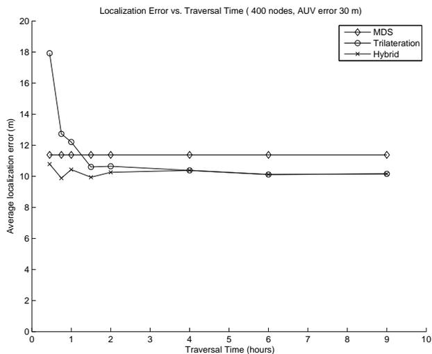
Figure 2. Localization Error (sparse networks)
