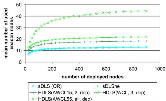
Figure 18. Mean number of used beacon nodes of best performing HDLS approaches for different limits of virtual beacon nodes
