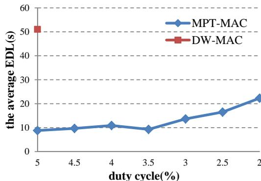
Fig. 14: Average EDL of MPT-MAC with different duty cycle
