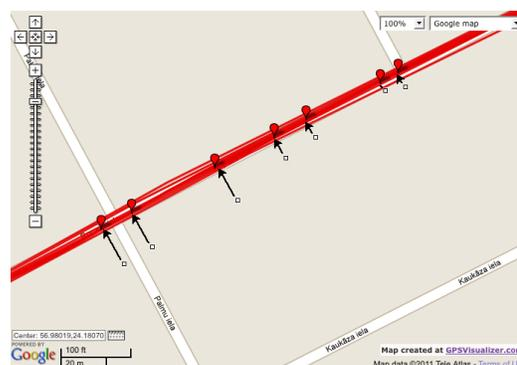
Figure 3. Manually marked ground-truth position improvement, by calculating perpendiculars to the test drive trajectory
