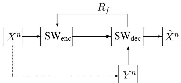
Figure 1. Rate-adaptive SW coding with a rate-limited feedback channel
