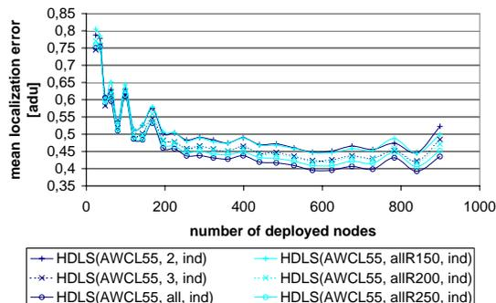
Figure 13. Range based equivalents of AWCL based HDLS approaches with independent distance estimation – mean localization error
