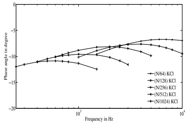
Figure 12. Experimental results showing shift in bandwidth of constant phase angle and change in ' $\alpha$ ' value with concentration change of KCl solution for FOE5
