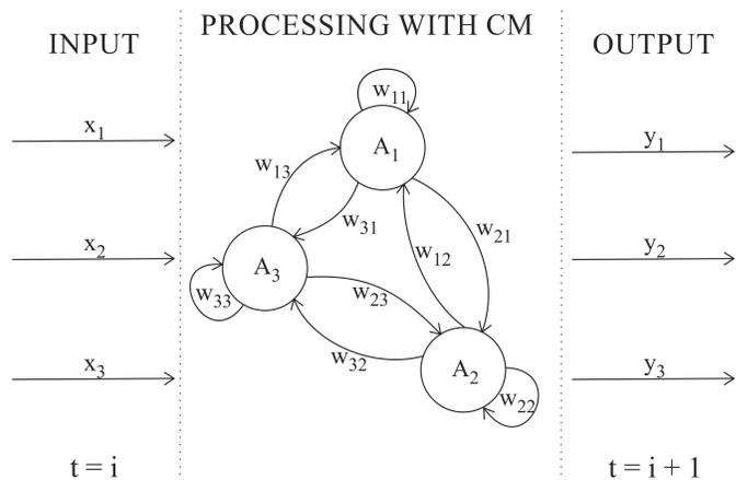
Fig. 1. Processing with a Cognitive Map (CM) with three nodes.
