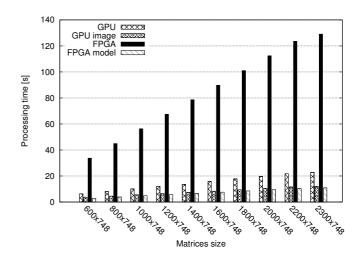
Figure 4. Results comparing available FPGA and GPGPU implementations.
