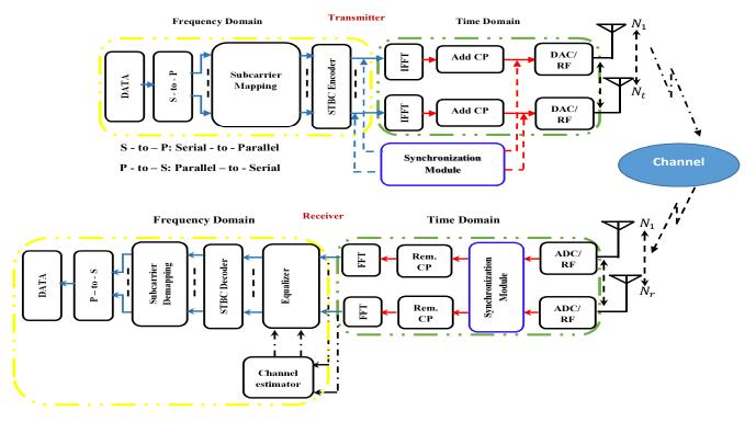
Figure 1. Transmission system MIMO-OFDM-STBC
