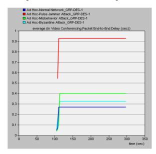
Figure 4. Packet end-to-end delay results of the normal network's video conferencing with and without network attacks for GRP
