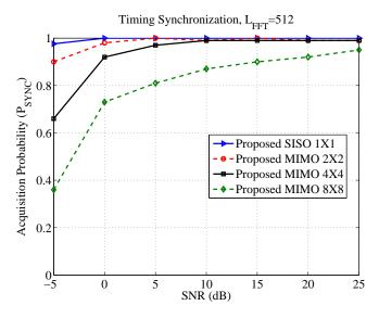
Figure 6. Timing synchronization performance of the proposed method  $\left( L_{FFT}=512\right)$
