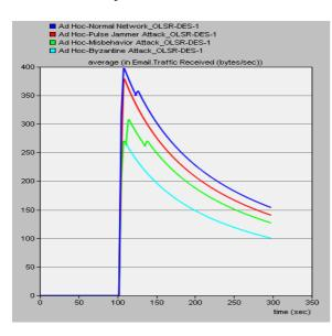
Figure 3. Traffic received results of the normal network's email application with and without network attacks for OLSR protocol
