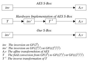
Figure 1. Structures of the different S-boxes in this paper.
