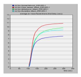
Figure 1. Packet end-to-end delay results of the normal network's voice application with and without network attacks for DSR
