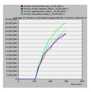
Figure 8. Data dropped results of the normal network with and without network attacks for OLSR
