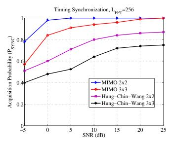
Figure 7. Comparisons between the proposed approach and subband-based preamble [10]
