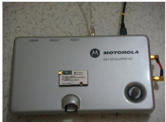
Figure 3. Motorola G24 Developer Kit (exterior)
