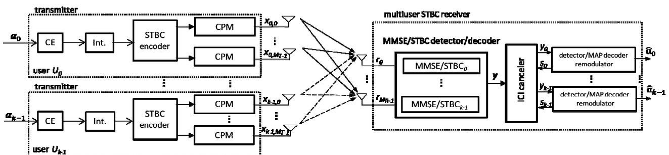
Figure 4. Block diagram of the analyzed CPM system.
