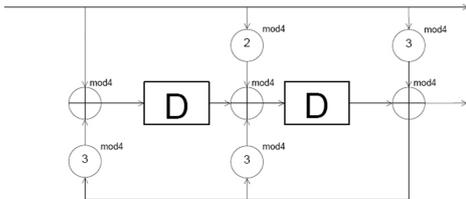
Figure 3. The systematic convolutional encoder over ring  $\mathfrak{R}=Z_4$ .
