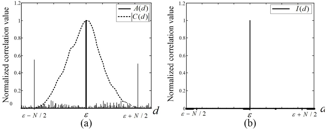
Figure 1. (a)  $A(d)$  and  $|C(d)|$  in the absence of channel distortion. (b)  $I(d)$  in the absence of channel distortion.
