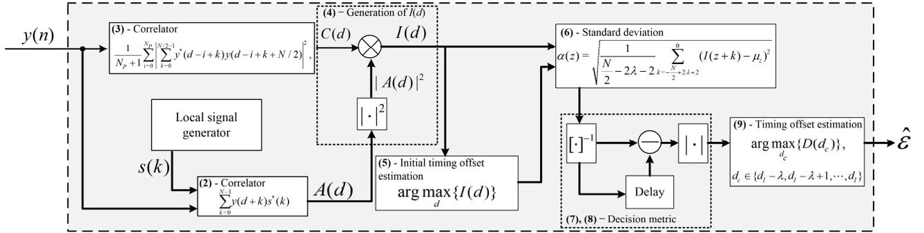
Figure 4. The overall structure of the proposed timing estimator.
