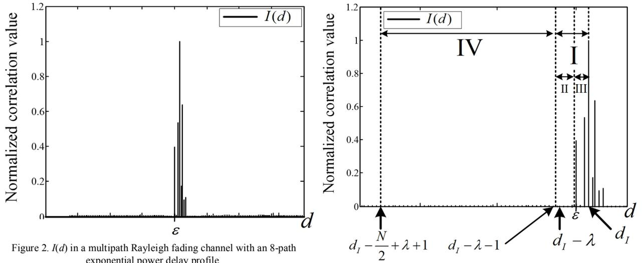
Figure 2.  $I(d)$  in a multipath Rayleigh fading channel with an 8-path exponential power delay profile.
