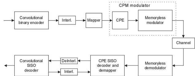
Figure 1. Serially concatenated convolutional encoder CE and CPM modulator.
