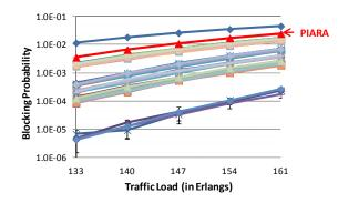
Figure 4. Blocking probability of all feasible shortest route combinations (M=64) of the R6NTL/IT=2 scenario.
