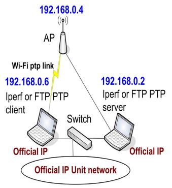
Figure 1. Laboratory setup scheme.
