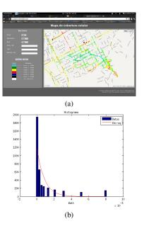
Figure 2: (a) Sample map of the cellphone coverage in Concepción, Chile. (b) Fitted and theoretical RSSI curves.
