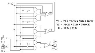
Figure 4. Intern aspect of the block Pv
