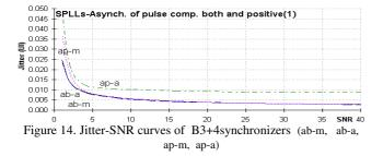
For prefilter B3=1.tx, we verify that, it becomes the jitter-SNR curves still more similar between themselves. For high SNR, it harms more the jitter-SNR curves. However, for low SNR, it benefits less the jitter-SNR curves.
