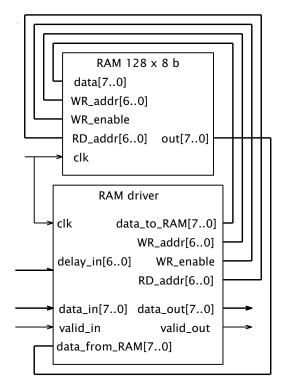
Figure 5. Delay block interconnection.
