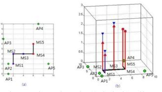
Figure 5. Experiment result comparison: (a) MS path and AP position distribution. (b) Comparison of positioning error adopting DOP and positioning error without adopting DOP.
