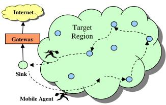
Figure 2. Mobile agent-based wireless sensor network
