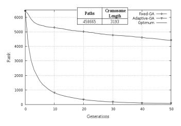
Fig. 6. Comparison between fixed-GA and adaptive-GA in dense networks
