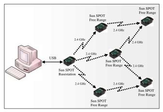
Figure 1. Wireless sensor network architecture
