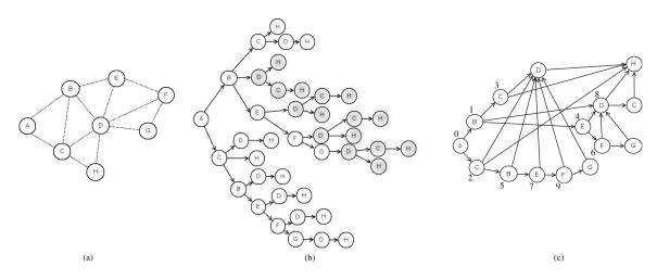
Fig. 1. (a) MANET example; (b) Tree network for source A and destination H; (c) Reduced tree network.
