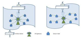
Figure 1. Underwater optical wireless network architecture
