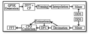
Figure 1. Baseband and IF transceiver arquitecture
