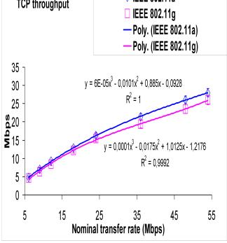
Figure 5. TCP throughput (y) versus technology and nominal transfer rate (x). Open links.
