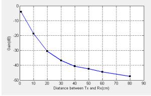
Figure 5. Link gain in different communication range
