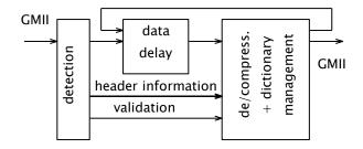
Figure 4. Block diagram of the de/compressor.
