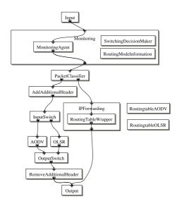
Fig. 3. Block Diagram of the Adaptive Routing Framework
