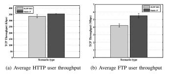
Fig. 5. TCP download throughput experienced by FTP and HTTP users
