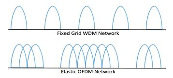
Figure 1. Comparing the spectrum of a WDM network with its fixed grid and that of an OFDM network with overlapping subcarriers.
