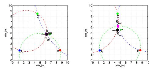
(a) experiment #3: actual position:  $(\hat{x}, \hat{y}) = (6.20, 4.72)$ , (b) experiment #4: actual position:  $(\hat{x}, \hat{y}) = (4.50, 5.50)$ ,  $err_{xy} = (-0.03, -0.01)$ ,  $err_{tot} = 0.03$ ,  $ori_{err} = 4$   $err_{xy} = (0.08, 0.69)$ ,  $err_{tot} = 0.69$ ,  $ori_{err} = 6$
