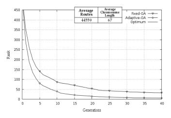
Fig. 11. Comparison between fixed-GA and adaptive-GA for a network with 40 nodes
