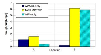
Figure 4. Total Throughput using MPTCP
