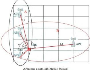
AP(access point), MS(Mobile Station) L1: line between AP1 and MS L3: line between AP3 and MS Lh: horizon line a2: angle between L3 and Lh a3: angle between L4 and Lh
