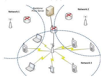
Figure 2. Multicast streaming scenario for a group of mobile clients switched to one mobile network after regrouping.
