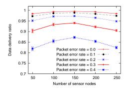
Figure 4. Data delivery ratio vs node density
