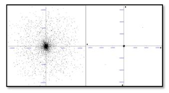
Figure 5. OFDM symbol with a 6 kHz offset between oscillators. Before compensation (left) and after compensation (right).
