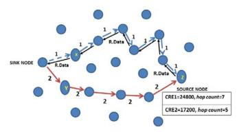
Figure 5. Illustration of the proposed CRE method. The Reinforcement and Reinforced Data propagation stages of the algorithms are shown.
