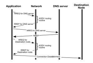
Fig. 1. Message sequence chart of connection establishment with reactive routing protocol
