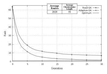
Fig. 10. Comparison between fixed-GA and adaptive-GA for a network with 30 nodes
