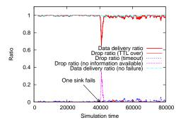
Figure 7. Data delivery ratio and drop ratio (sink node failure)
