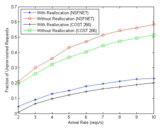
Figure 4. Comparing the routing and spectrum assignment algorithm for tight deadlines with and without the reallocation phase
