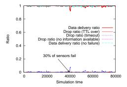
Figure 5. Data delivery ratio and drop ratio (sensor nodes failure)
