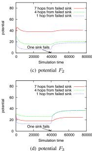
Figure 6. Potential convergence after sink-node failure
