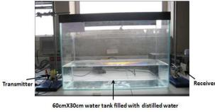
Figure 8. Water test setup
