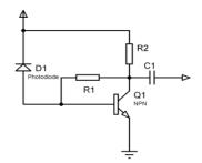
Figure 4. Modified transimpedance receiver front end
