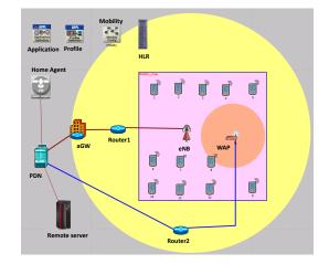
Fig. 3. Overview of the considered simulation scenario in the OPNET simulator. The large circular area shows the LTE network coverage and the smaller circular area shows the WLAN network coverage. The user movement is restricted to the rectangular area inside the large circle.
