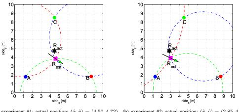
(a) experiment #1: actual position:  $(\hat{x}, \hat{y}) = (4.50, 4.72)$ , (b) experiment #2: actual position:  $(\hat{x}, \hat{y}) = (2.85, 4.72)$ ,  $err_{xy} = (0.11, -0.88)$ ,  $err_{tot} = 0.89$ ,  $ori_{err} = -35$   $err_{xy} = (0.13, -0.81)$ ,  $err_{tot} = 0.82$ ,  $ori_{err} = -25$
