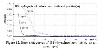
For prefilter  $B1=\infty$ , we verify that, for high SNR, the four synchronizer jitter-SNR curves tend to be similar. However, for low SNR, the variant asynchronous by both at rate with versions manual (ab-m) and automatic (ab-a) are better than the variant asynchronous by positive at rate with versions manual (ap-m) and automatic (ap-a).
