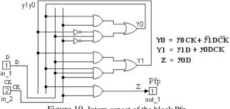
Figure 10. Intern aspect of the block Pfp
