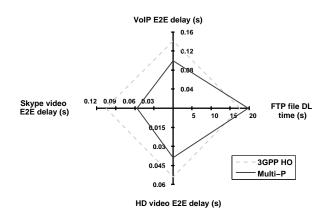
Fig. 2. End-to-end delay comparison spider web graph
