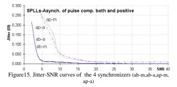
We observe that, in general, the output jitter UIRMS decreases gradually with the input SNR increasing.
