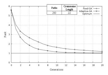
Fig. 5. Comparison between fixed-GA and adaptive-GA in sparse networks
