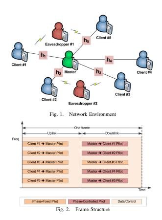
Since the pilot signal is controlled only during key generation period, phase-controlled pilot does not affect equalization or AMC scheme. Other resource except pilot signal is utilized to transmit data or control signal. It is assumed wireless channel response is quasi-static during key generation and thus users can exploit channel reciprocity.
