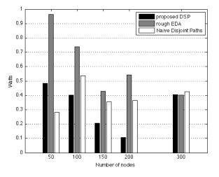
Figure 3. Average power dissipated in retransmissions.
