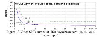
For prefilter B2=2.tx, we verify that, it becomes the jitter-SNR curves more similar between themselves. For high SNR, it degrades slightly the jitter-SNR curves. However, for low SNR it benefits significantly the jitter - SNR curves.
