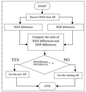
Figure 4. The proposed positioning algorithm.
