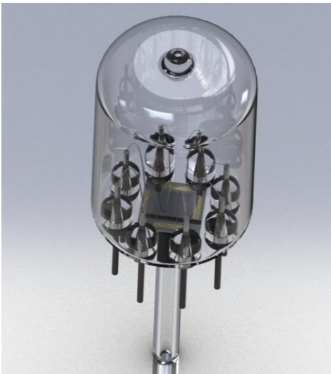
Figure 10. Possible package for emitter made from carbon nanotubes.
